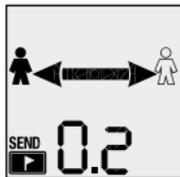
In case a regular group check is impossible due to limited space, it is possible to perform a basic verification if the transceivers of all participants are turned on.
