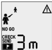
If your Barryvox® detects that the transmit frequency of the tested device is out of tolerance, a warning message will be shown. Such devices must be checked by the manufacturer.
