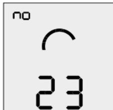
As soon as the “Maintenance” screen is shown, press and hold the
