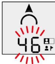
If the signal of the buried subject you are currently searching for temporarily overlaps with another signal, the device tries to guide you along the optimal search path. If the signals overlap for a long period of time, reliable guidance is limited. The device indicates this with a flashing distance indication. Radically slow the search until the distance indication stops flashing, indicating the signal overlap has cleared.
