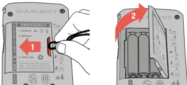
Use a fingernail or the leash clip to slide battery door to the left, and it will swing open.
