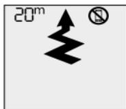
Reduced signal search strip width due to interference.
