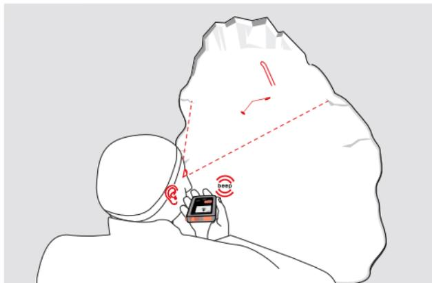
The avalanche surface is searched systematically until you pick up a signal. During the acoustic signal search, the rescuer has the visual focus on the surface of the debris in order to be able to see body parts or objects protruding the snow surface.
