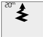
Reduced signal search strip width due to a device transmitting outside the standard frequency.
