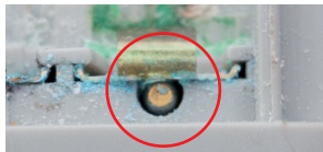
A contaminated main battery connector
