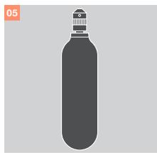
**CAUTION:** Screw the cartridge in completely (the black rubber seal must not be visible). The cartridge must be secured using velcro.
